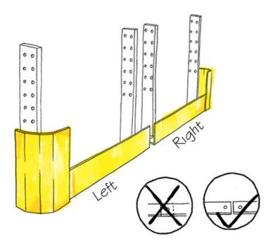
Simply anchor the rack pals to the floor. Cogan recommends to always install on a concrete surface.
